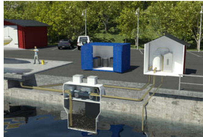
Cleaning effluent: Collection and settling
